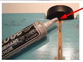
Step 2: Squeeze tube gently to apply small amount of graphite into back of wheel hub
