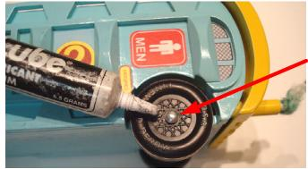
Step 1: Squeeze tube gently to apply small amount of graphite under axle head
